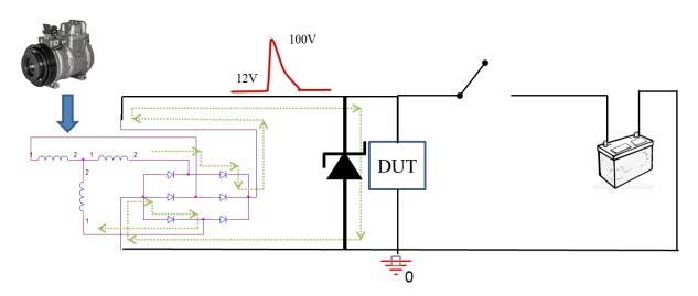
Figure 2. ISO 16750-2 Load dump Test A
