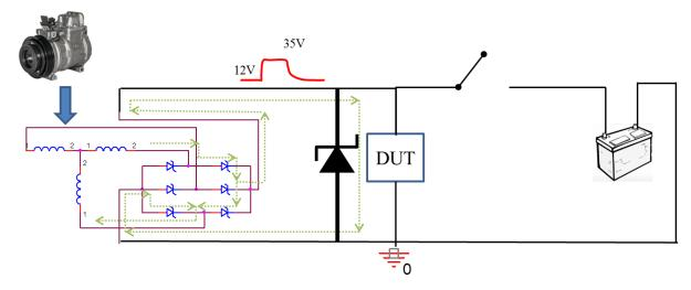
Figure 3. ISO 16750-2 Load dump Test B
