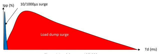
Figure 1. Load dump vs. 10/1000μs surge energy
