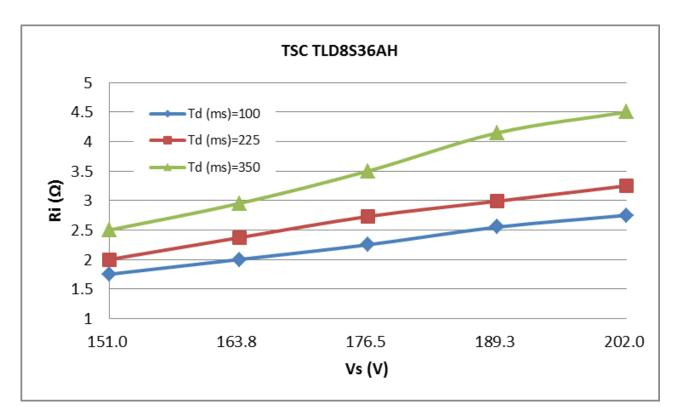
Figure 5. TLD8S36AH SOA (ISO 16750-2 Load dump Test A) Test A
